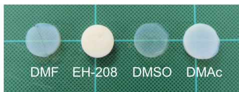
Fig. 7 Examples of transparent aerogels from BTMPA prepared through a one-step base process in different solvents; DMF, EH-208, DMSO, and N,N -dimethylacetamide (DMAc)
