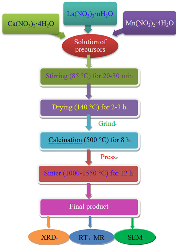
Fig. 1 Flow diagram of Sol-gel method used to synthesize high grade LCMO polycrystalline ceramics
