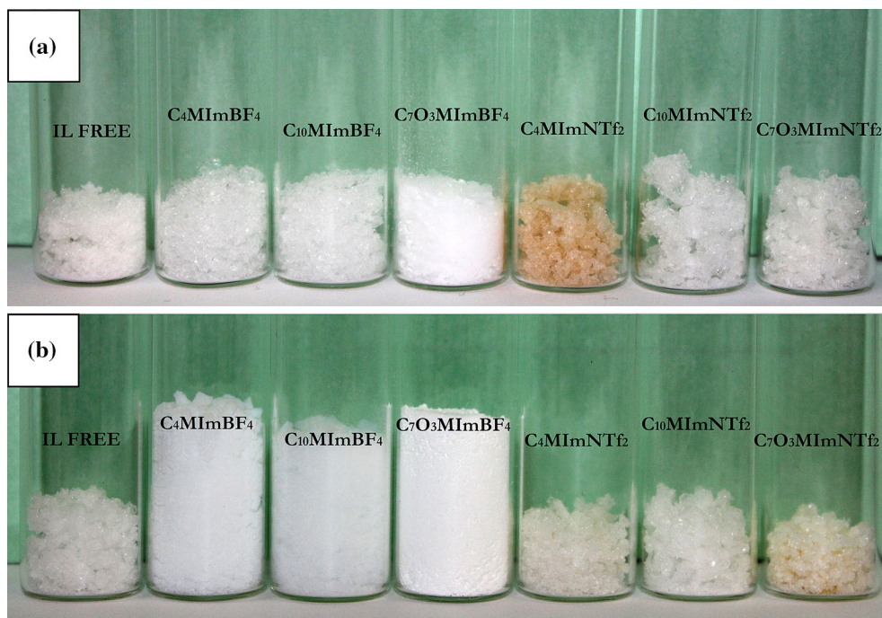
Fig. 3 Comparison of 1 g non-grinded silica xerogels synthesized under identical conditions at either RT (a) or 60 °C (b), varying only the IL applied. From the left to right : IL-free, C 4 MImBF 4 , C 10 MImBF 4 , C 7 O 3 MImBF 4 , C 4 MImNTf 2 , C 10 MImNTf 2 and C 7 O 3 MImNTf 2
