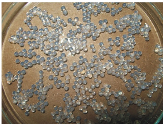
Fig. 1 Photograph of general beads formed by simple ionic gelation
