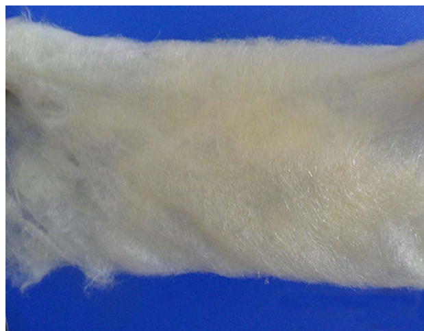
Fig. 2 Optical image of Ti(CH 3 COO) 4 precursor fibers
