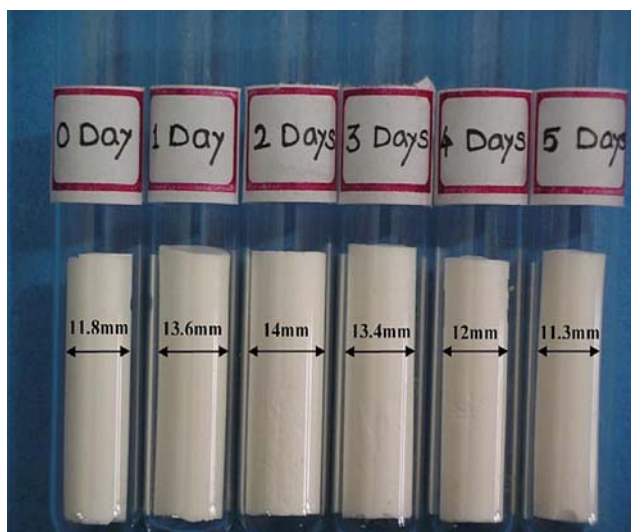
Fig. 3 Photograph showing the shrinkage in the volume of aerogel samples at various aging period
