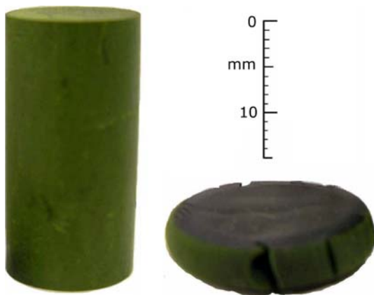
Fig. 8 X-VOx samples before ( \rho_b = 0.420 g/cm 3 ) and after ( \rho_b = 1.024 g/cm 3 ) quasi-static compression testing
