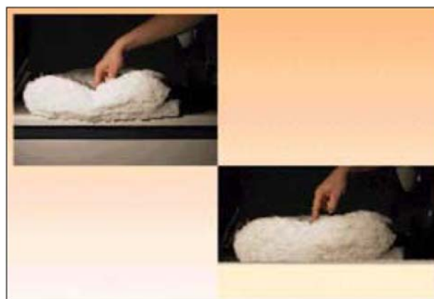
Fig. 17 Elastic glass fiber mats with highly inorganic sol-gel binders
