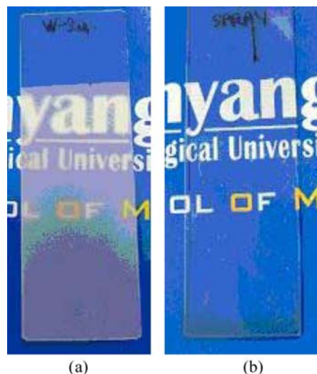
Figure 3. Photographs of HAC catalysed (HAC:TIP:PDMS = 0.125:1:2) translucent (a) and EAcAc modified (TIP:EAcAc:PDMS = 1:2:2) transparent (b) glass slides using only the TIP/PDMS solutions (no MTES/TEOS nor silica filler is added). Coatings are cured at 200°C for 90 min.
