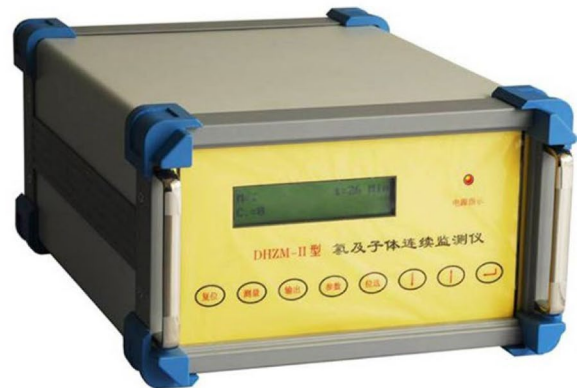
DHZM-II radon monitor
