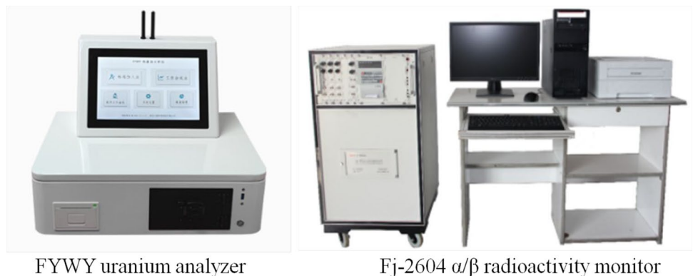
Fig. 7 Instruments used for measuring total uranium, gross \alpha and gross \beta
