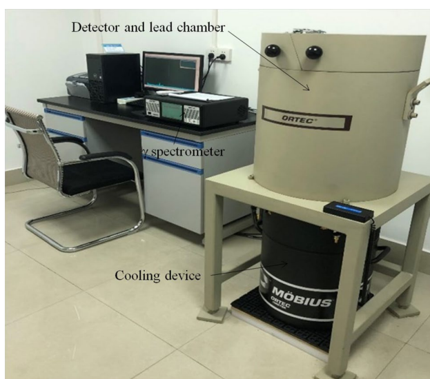
Fig. 5 GEM HPGe \gamma spectrometer
