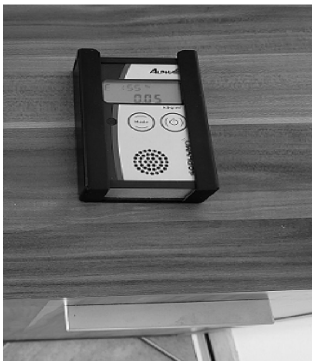
Fig. 2 AlphaE radon meter placed in investigation location
