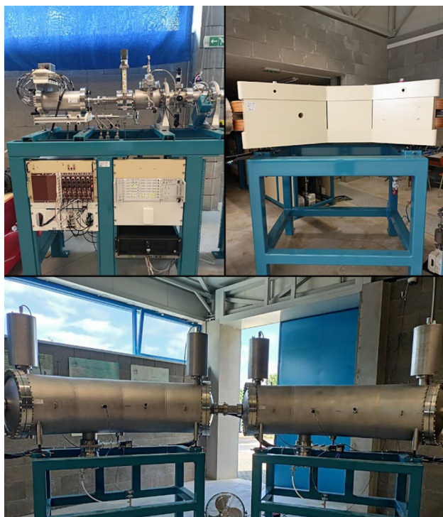
Fig. 4 Newly installed AMS parts of the tandem accelerator system at the CENTA laboratory: 4-anode ionization chamber (top left), high-resolution analyzing magnet (top right), and two electrostatic analyzers (bottom)
