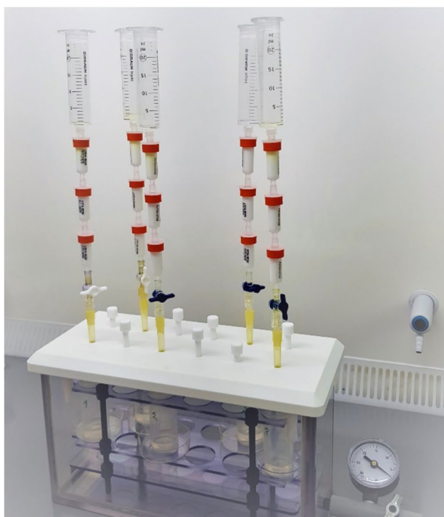
Fig. 5 3-stage separation columns to remove the uranium matrix from the sample solutions
