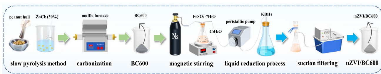
Fig. 1 The process diagram of synthesis nZVI/BC600 in this experiment
