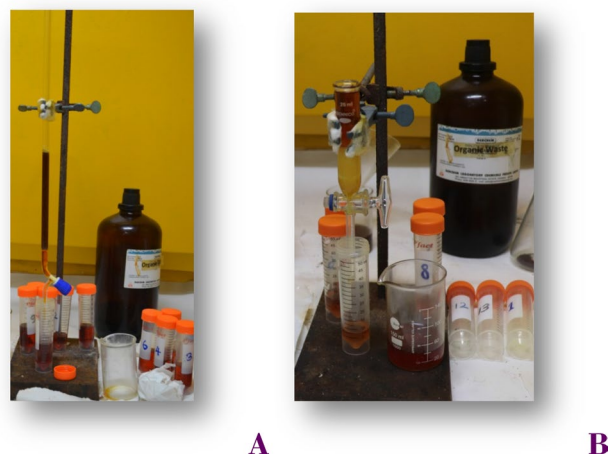
Fig. 2 Column demonstration of the organic waste treatment by PS-DVB-DGAH (A) and solid state complexant (B)
