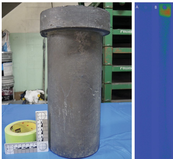
Fig. 3 Left—photograph of the as-cast depleted uranium rod after breakout and cleaning. Right – A: Radiograph collected on the exterior of the depleted uranium metal rod; B: Radiograph collected on the interior of the depleted uranium metal rod. Both radiographs were produced from a 5-min exposure of the metal to the imaging film. Radioactivity is shown by an increase in warm colors of each pixel (towards red). An increase in radioactivity near the upper portion (hot top) of the casting is visible primarily in the interior film radiograph. Background radiation/exposure is shown in blue. Radioactivity intensity scales from green (low) to (red) and is qualitative rather than quantitative
