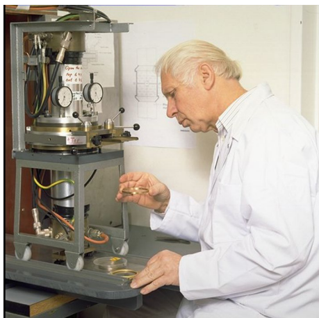
Fig. 1 The 4\pi CsI(Tl) sandwich spectrometer with surrounding lead shield. Designer of the instrument, Bruno Denecke, holding a bespoke source support
