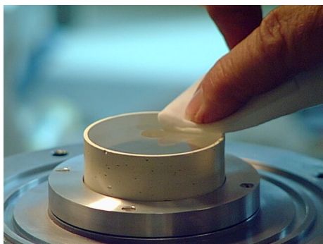
Fig. 2 Shape of a CsI(Tl) crystal (51 mm diameter, 25 mm height) with a semi-spherical cavity in its surface that will surround the radioactive spot
