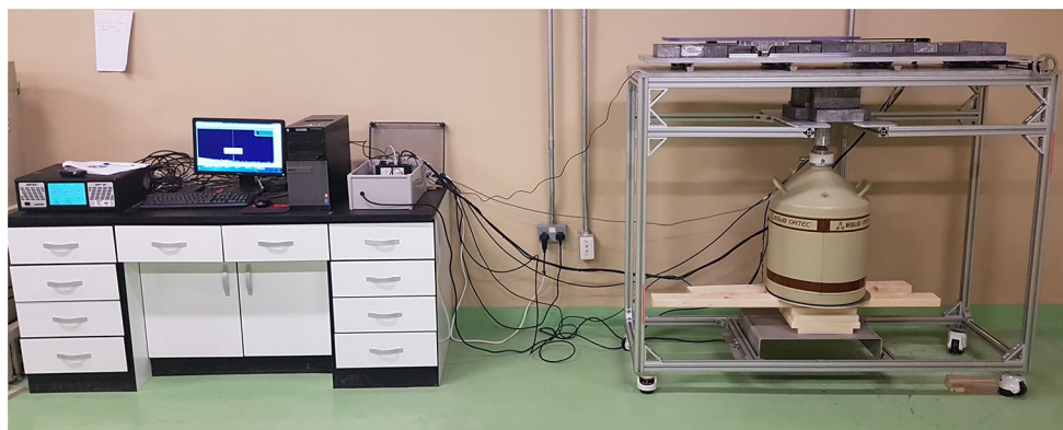
Fig. 5 The installed wire scanning system
