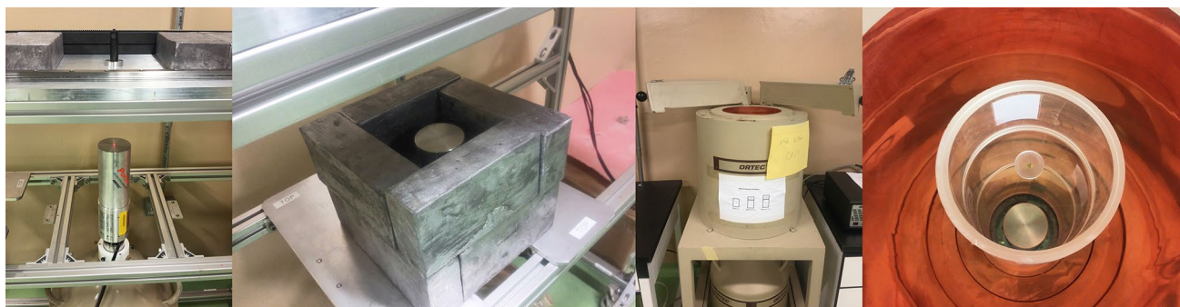
Fig. 6 HPGe detectors installed in the wire scanning system and in the low-background shield
