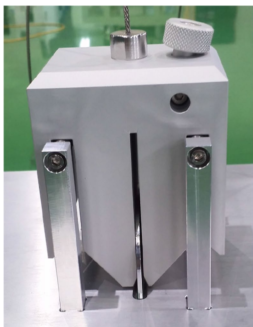
Fig. 2 Picture and 3D model of the tool used to withdraw the detector mount from the fuel assembly
