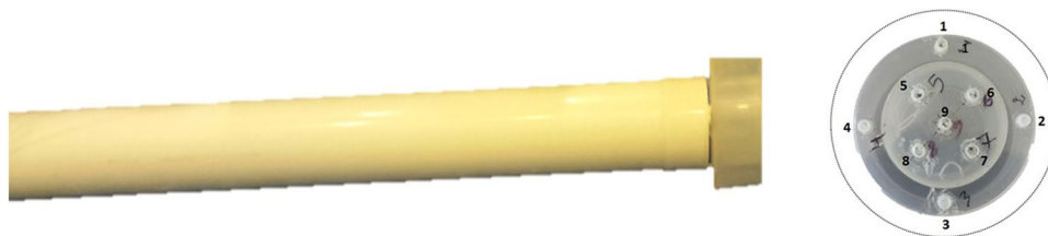
Fig. 1 On the right: PS with nine front-sealed PE vials used to contain the activation detector foils; on the left: the experimental assembly for inserting the PS into the beam tube
