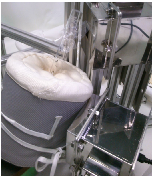
Fig. 3 Side view of the experimental setup without using a thermoelectric cooler for dry distillation
