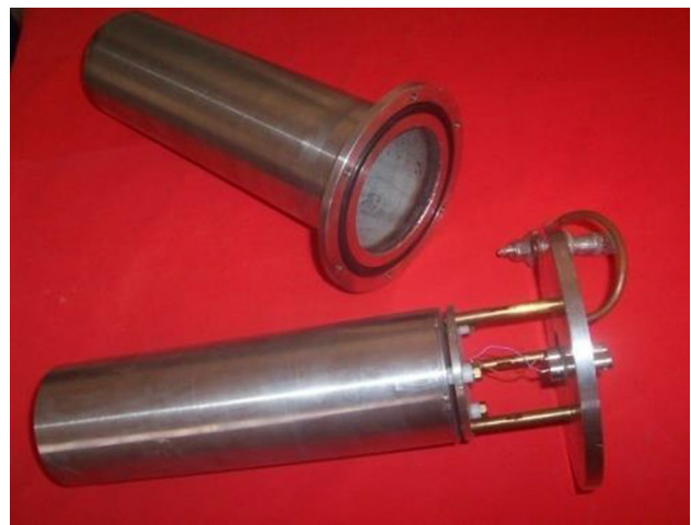
Fig. 9 Picture of versatile gamma ionization chamber prototype (VGIC) [8], [15]
