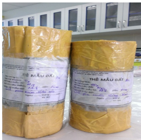
Fig. 2 Soil cores taken from the steel tube sampler
