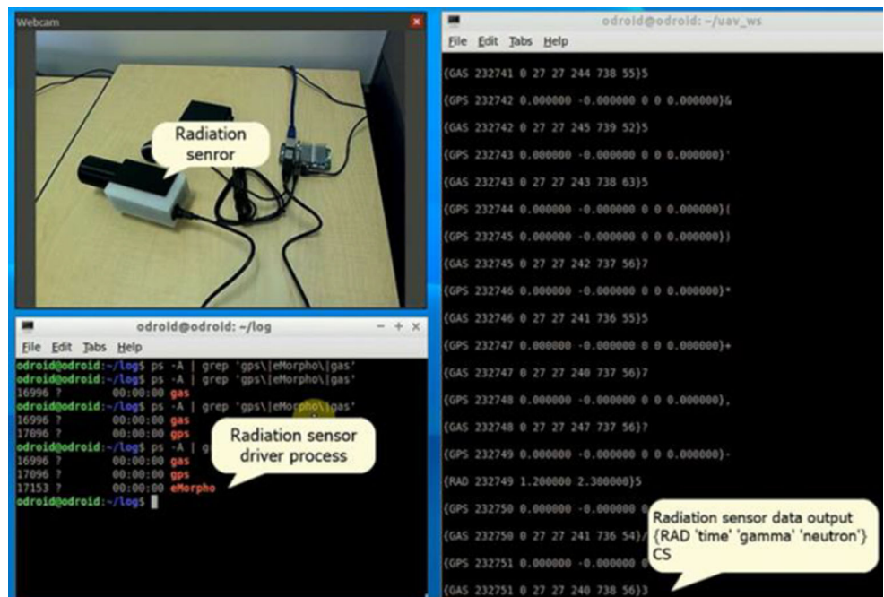
Fig. 6 Test of the plug-and-play operation of a CLYC sensor
