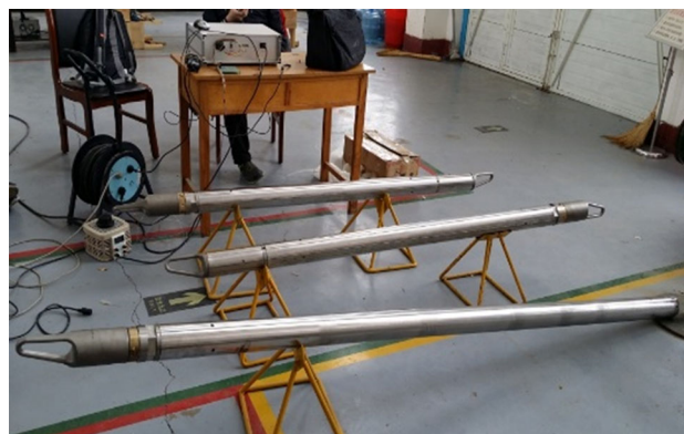
Fig. 12 Picture of the pulsed neutron well logging instrument
