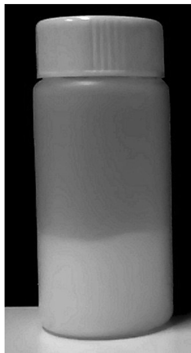
Fig. 2 Scintillation vial filled with the PSm and the active solution ready to be measured
