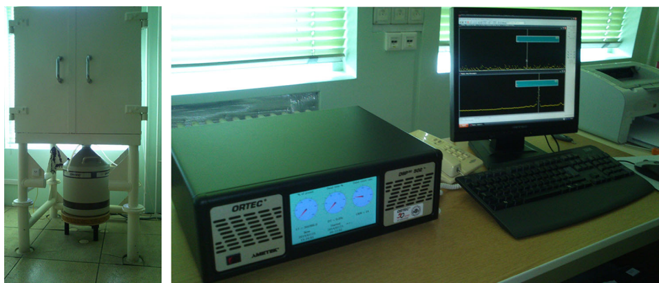
Fig. 2 The new counting station “D5” with the ORTEC DSPEC 502 dual input digital spectrometer
