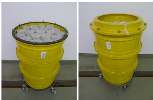
Fig. 1 200 L steel drum filled with concrete blocks (left) and closed with the cover (right) before loading in the MEDINA facility
