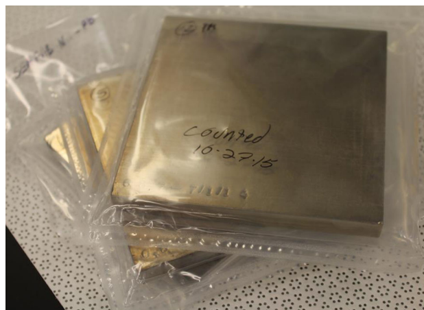
Fig. 1 Lead samples prepared in a standard geometry for calibrating the equivalent 210 Pb concentration based on a \gamma -ray measurement of 210 Bi bremsstrahlung spectrum
