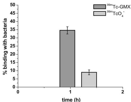
**Fig. 7** In vitro binding of <sup>99m</sup>Tc-GMX with *E. Coli* in comparison with <sup>99m</sup>TcO<sub>4</sub><sup>-</sup> 1 h after incubation at 4 °C
