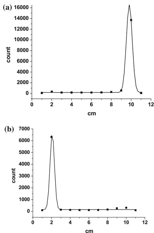
**Fig. 4** TLRC chromatograms of  $^{99m}\text{Tc}$ -GMX developed in ethanol:water:ammonium hydroxide (2:5:1 v/v) with  $^{99m}\text{Tc}$ -GMX in  $R_f = 1$  and  $^{99m}\text{TcO}_2$  in  $R_f = 0$  (a) and in acetone solvent with  $^{99m}\text{Tc}$ -GMX in  $R_f = 0$  and  $^{99m}\text{TcO}_4^-$  in  $R_f = 1$  (b).  $^{99m}\text{Tc}$ -GMX showed  $98.60 \pm 0.70$  % labeling yield
