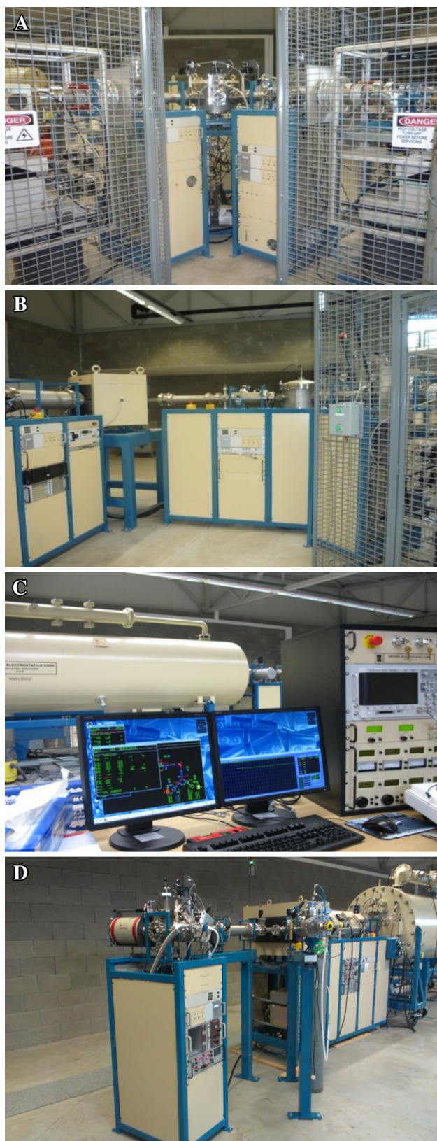
Fig. 2 View of the main components of the tandem laboratory. a Alphasource (left) and MC-SNICS ion sources (right); b Injection line; c Pelletron accelerator with control system; d Ion analyzer with switching magnet and ion beam lines
