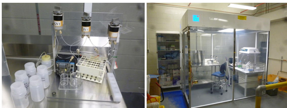
Fig. 3 GPEC apparatus ( left ) set up in the class 1000 clean room ( right )
