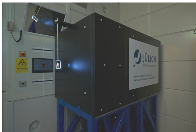
Fig. 5 FaNGaS, the fast neutron gamma spectroscopy instrument at the SR10 beam line of FRM II Research Reactor in Garching
