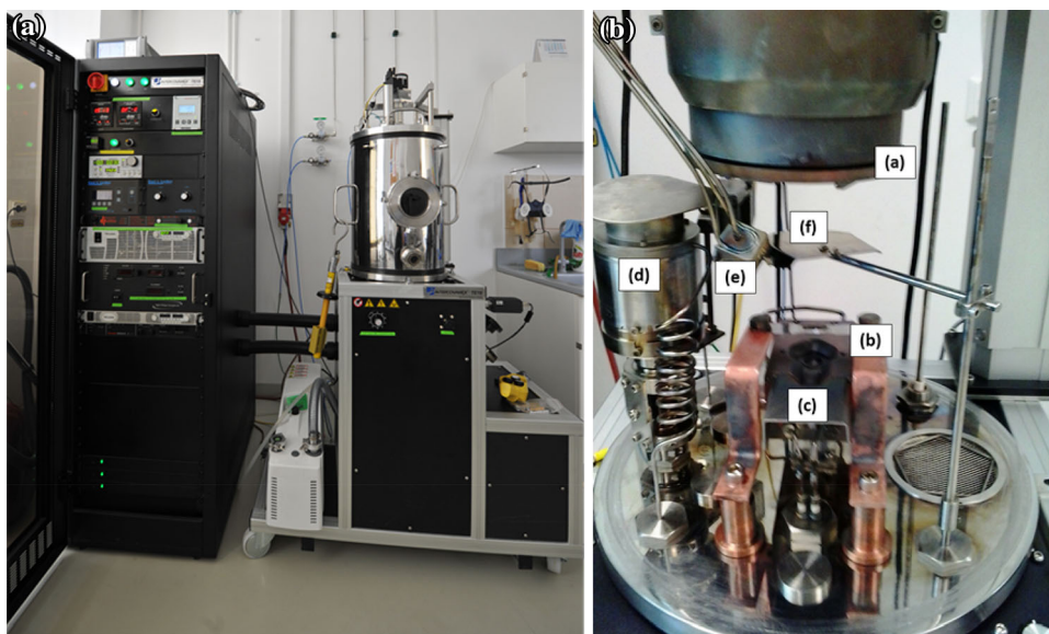
Fig. 2 A TE18-High Vacuum Deposition System produced by Intercovamex Company; B interior of the deposition chamber, showing: a rotating substrate holder; b thermal evaporation; c electron-beam evaporation system; d sputtering deposition system; e quartz crystal monitor; f shutter
