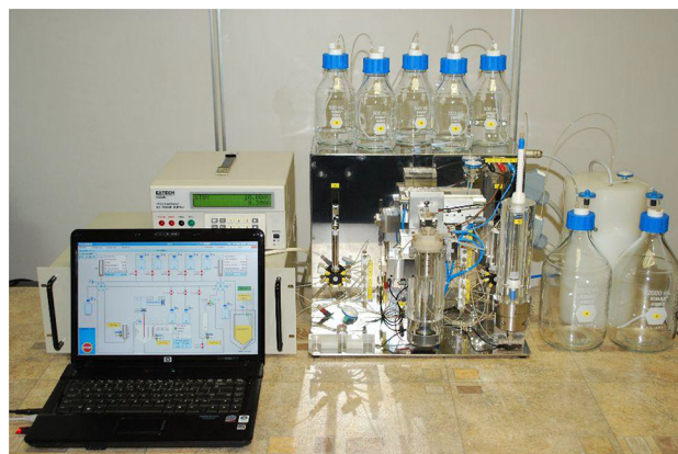
Fig. 2 Kamadhenu, ^{90}\text{Sr}/^{90}\text{Y} electrochemical generator (courtesy of Dr. Josef Comor). The electrochemical cell, ^{90}\text{Sr} storage container, reagent solution vessels, waste solution collection vessel, etc., are illustrated together with the PC controlling the operations. The generator components and computer need to be housed in a hot cell
