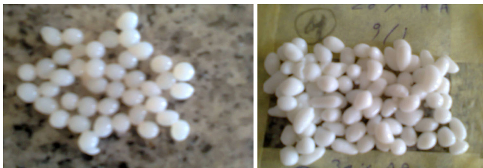
Fig. 1 Photographs of (ALG/Chit) gel beads before and after grafting with AAC
