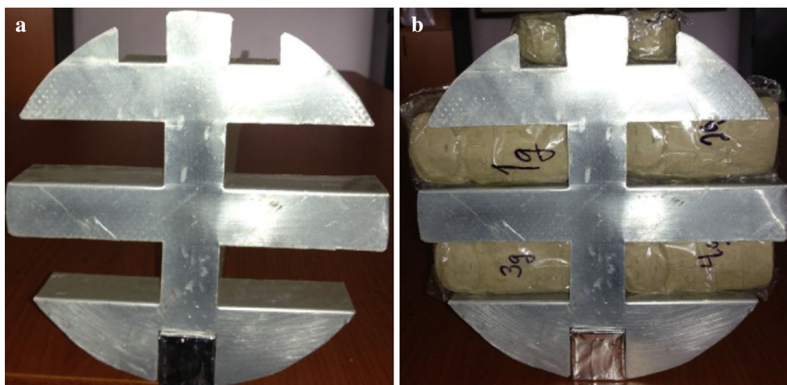
Fig. 1 Figurines sample arrangement for its irradiation inside the radial channel
