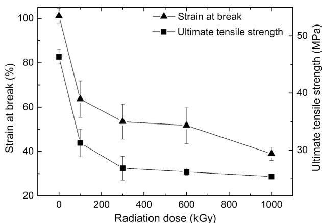
**Fig. 6** Changes in strain at break and ultimate tensile strength as a function of radiation dose
