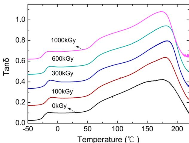
**Fig. 1** DMA spectra of polyurethanes irradiated at various dose
