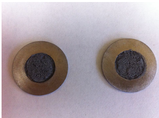
Fig. 3 ^{100}\text{Mo} -targets for the GE PETtrace cyclotrons
