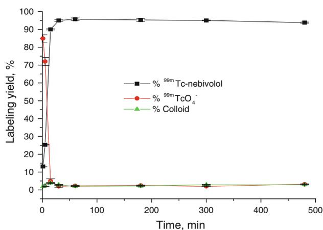
**Fig. 5** Radiochemical yield of  $^{99m}\text{Tc}$ -neбивол as a function of reaction time  $^{99m}\text{Tc}$ -neбивол yields versus reaction time; reaction conditions:  $200 \mu\text{g}$  neбивол,  $200 \mu\text{g}$  of  $\text{SnCl}_2 \cdot 2\text{H}_2\text{O}$ ,  $1.0 \text{ ml}$  ( $\sim 195 \text{ MBq}$ ) of  $^{99m}\text{TcO}_4^-$  at pH 6, the reaction mixture was kept at room temperature for different intervals of time
