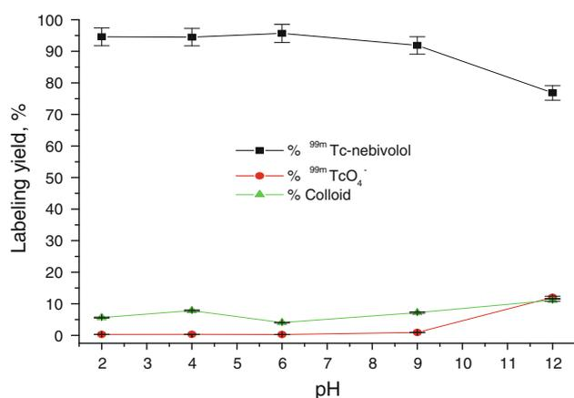
**Fig. 6** Radiochemical yield of <sup>99m</sup>Tc-nebivolol as a function of pH Effect of pH on the labeling yield of nebivolol; reaction conditions: 200 μg nebivolol, 200 μg SnCl<sub>2</sub>·2H<sub>2</sub>O, 1.0 ml (~195 MBq) of <sup>99m</sup>TcO<sub>4</sub><sup>-</sup> at pH = x, the reaction mixture was kept at room temperature for 30 min
