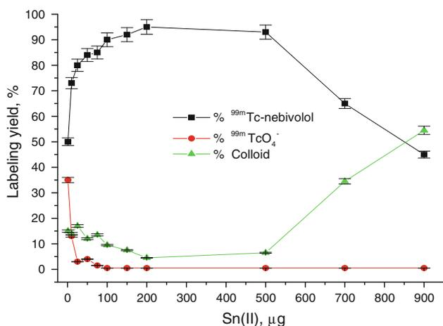
**Fig. 4** Radiochemical yield of  $^{99m}\text{Tc}$ -neбивол as a function of reducing agent amount. Effect of  $\text{SnCl}_2 \cdot 2\text{H}_2\text{O}$  concentration on the labeling yield of  $^{99m}\text{Tc}$ -neбивол; reaction conditions:  $200 \mu\text{g}$  neбивол,  $x \mu\text{g}$  of  $\text{SnCl}_2 \cdot 2\text{H}_2\text{O}$ ,  $1.0 \text{ ml}$  ( $\sim 195 \text{ MBq}$ ) of  $^{99m}\text{TcO}_4^-$  at pH 6, the reaction mixture was kept at room temperature for 30 min
