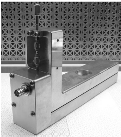
Fig. 1 The PNNL ultra-low background proportional counter. The cylindrical body of the detector is contained within a solid copper holder which provides additional shielding. A copper SHV enclosure (lower left region of figure), with a connector for applied bias, provides electrical shielding for the high-voltage penetration to the detector's inner volume. A double-valved assembly (extending vertically above the copper SHV enclosure) seals the detector's gas-fill capillary
