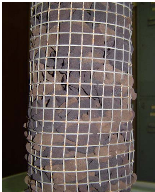
Fig. 2 Cartridge loaded with CFC-HMO PU foam
