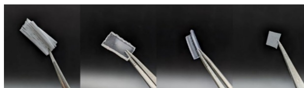
Fig. 13 From left to right: Samples of PMP, MABS, PVC, and PU used for FTIR-ATR measurements
