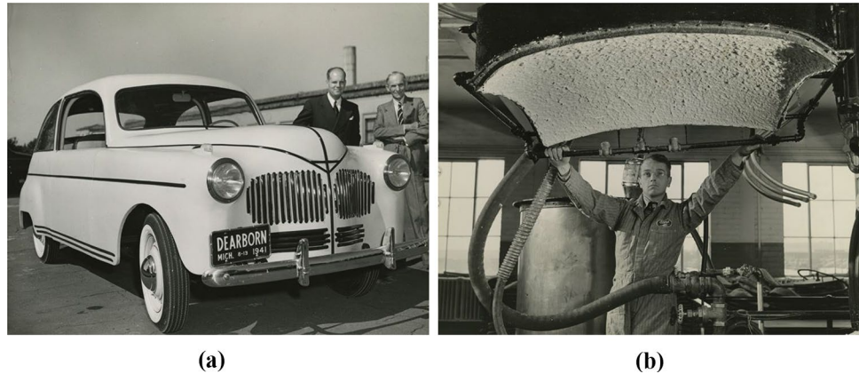
Fig. 2 a Ford experimental soybean car and b manufacturing of panel for soybean car [45]
