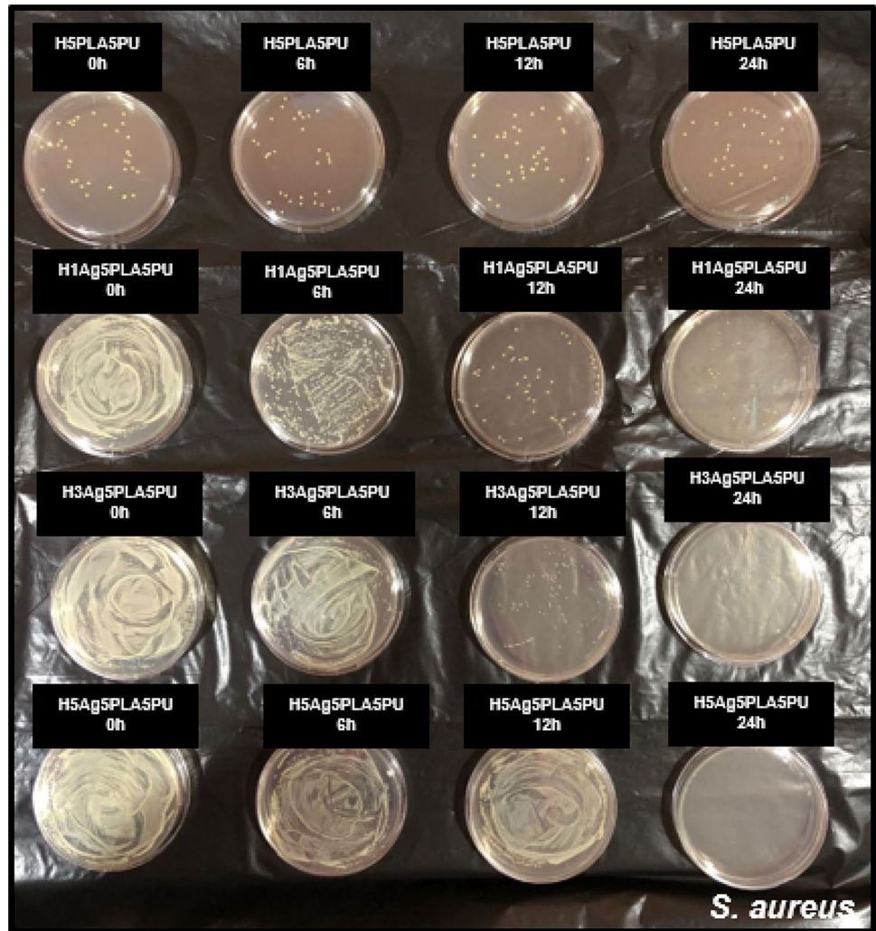
Fig. 11 Antibacterial effect of hollow PLA/PU/Ag NP nanofibers on S. aureus (from left to right: 0, 6, 12, 24 h, respectively) (from top to bottom, respectively: H5PLA5PU, H1Ag5PLA5PU, H3Ag5PLA5PU and H5Ag5PLA5PU)
