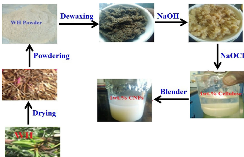
Fig. 1 Schematic representation of cellulose isolation and CNFs preparation from water hyacinth
