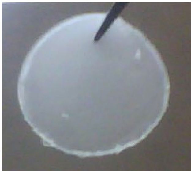
Fig. 1 Photograph of optimized gel polymer electrolyte film
