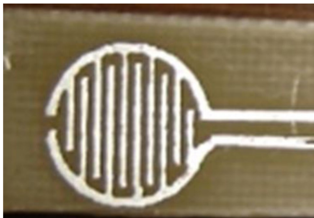
Fig. 2 Photo image of the simple, comb-like interdigitated electrode
