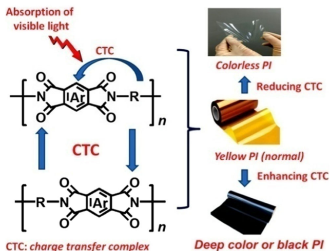
Fig. 1 Color tailoring of PI films by adjustment of CTCs
