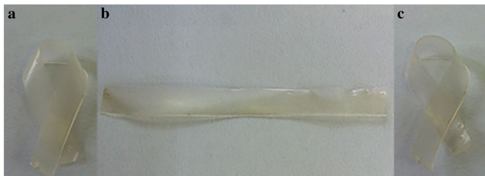
Fig. 6 Thermally induced shape-memory behavior of X(HPC-g-PCL) SMP films (with 4.8 cm length and 0.1 mm thickness) (a) Permanent shape (b) temporary shape fixed at 0 °C (c) the recovered shape after 10 s immersion in water at 39 °C
