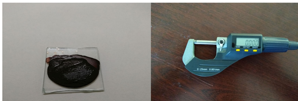
Fig. 1 Images of 106 \mu\text{m} coated poly(NIMP) film and micrometer
